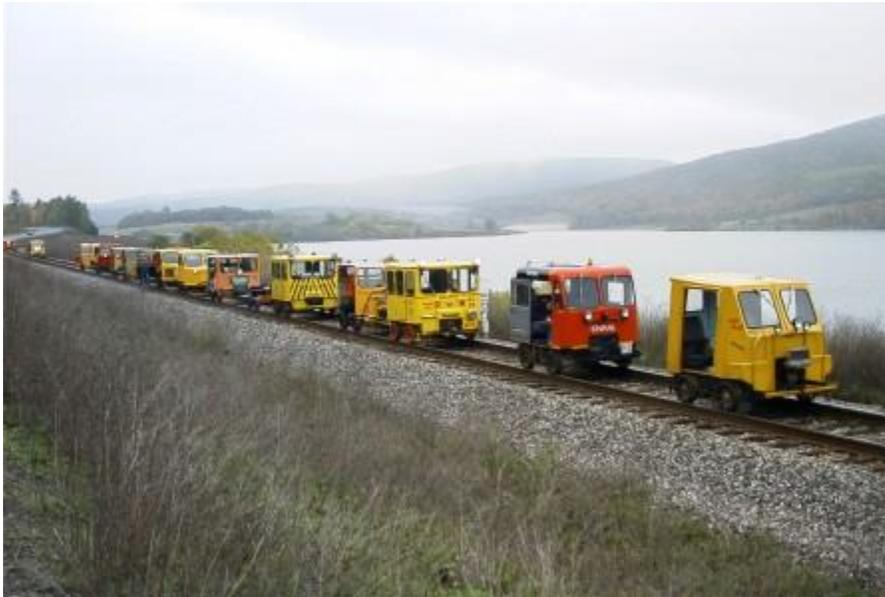
*Figure 2 We seek to convert to battery power a historic rail "speeder," a self-propelled, 4-wheel vehicle formerly used in maintenance of way service.*
